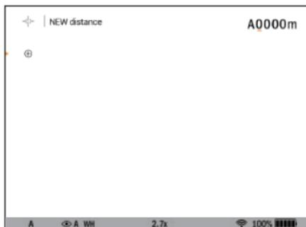
Press **Left/Right** Button and you will see **A0000m**, set the value for each digit with Press **Up/Down** Button, switch between the digits with a short press of **Left/Right** Button. Press **Middle** Button to save the new distance.
