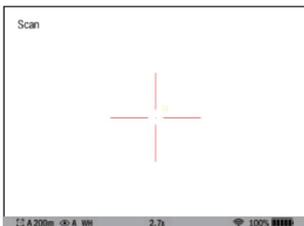
Distance to the object displays in status bar and a "
