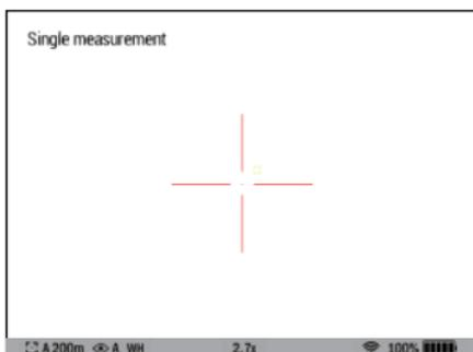
When under real time image mode, Long press **Down** Button to enter/exit scan mode. Aim
